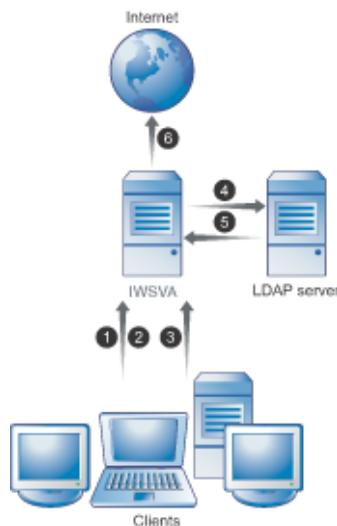
**FIGURE 7-1. LDAP Communication Flow Using Kerberos Authentication**
