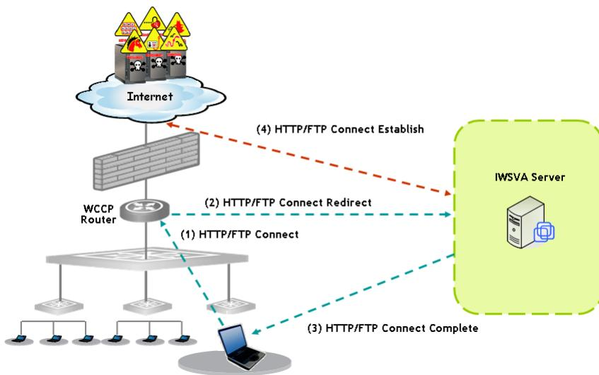
FIGURE 6-1. WCCP configuration and Web and FTP traffic
