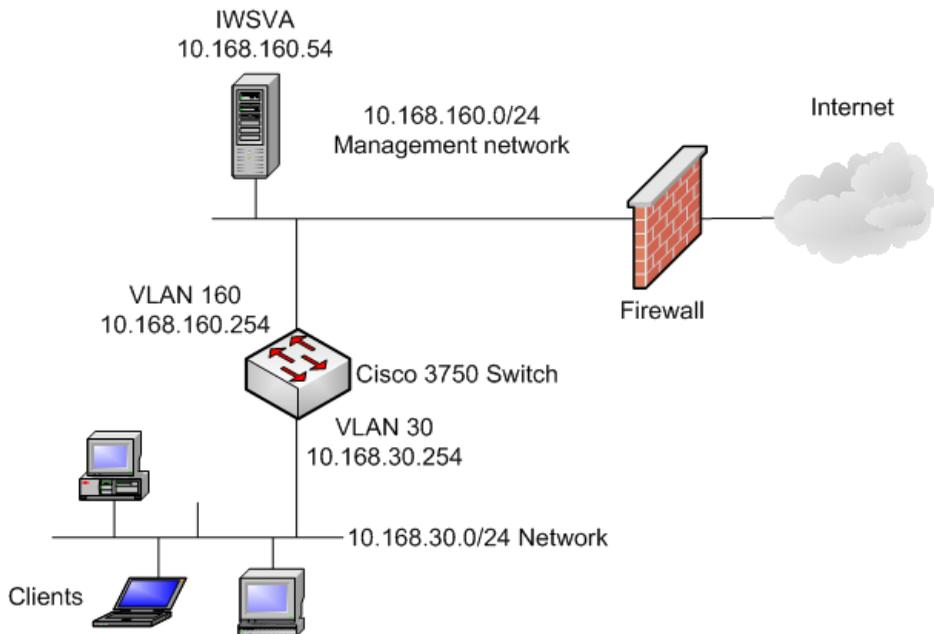
FIGURE F-2. Example Topology for Cisco 3750 Switch Implementation
