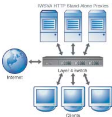
FIGURE 6-4. Forward proxy with transparency
