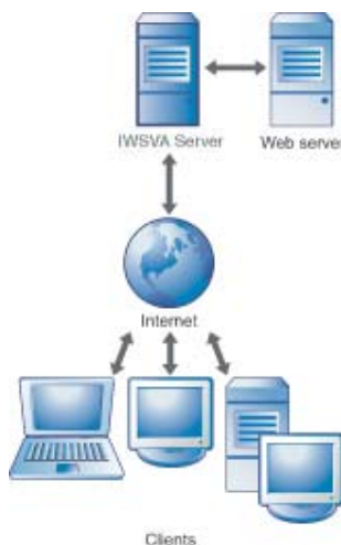
FIGURE 6-5. Reverse proxy protects Web server from clients
