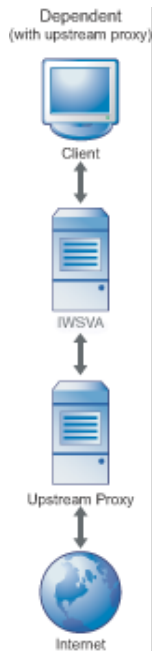
FIGURE 6-3. Forward, upstream proxy
