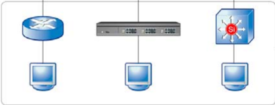
FIGURE 2-7. IWSVA deployment in a WCCP environment
