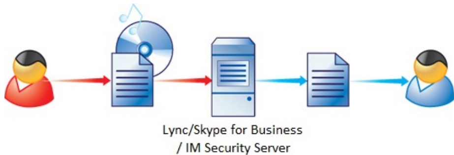
FIGURE 1-3. How IM Security File Blocking works
