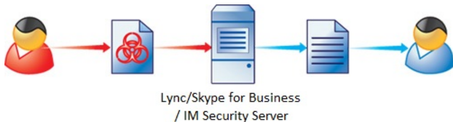
FIGURE 1-2. How IM Security Virus Scan works
