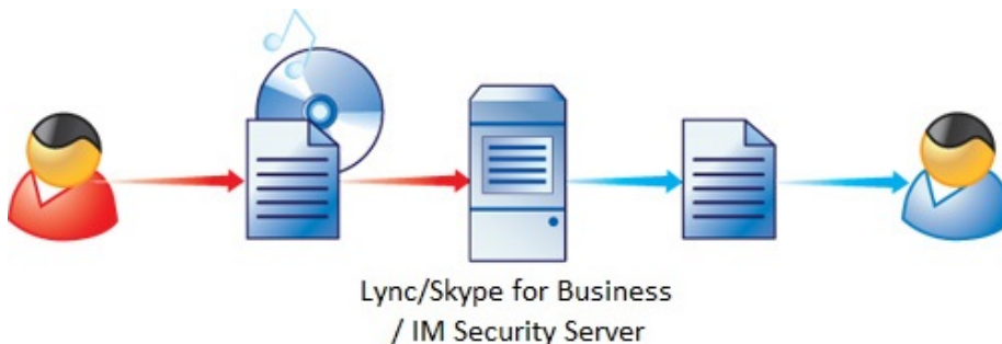
FIGURE 1-3. How IM Security File Blocking works
